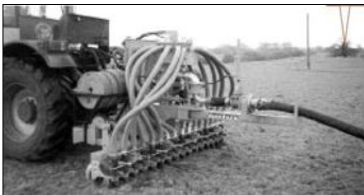
**Figure 2.42:** Example of an open-slot shallow injector
