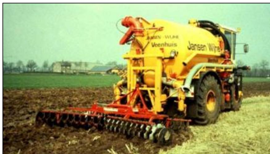
**Figure 2.43: Incorporation equipment combined with a big tanker**
