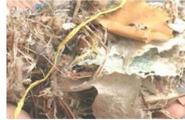
**Figure 1.9: Specially prepared household waste used as fuel in cement kilns**
