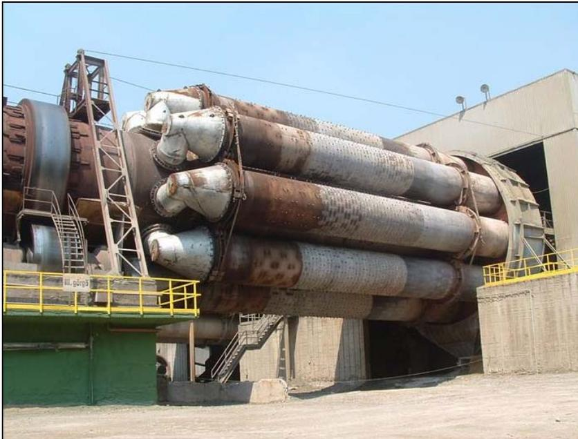
**Figure 1.18:** Example of a planetary cooler
