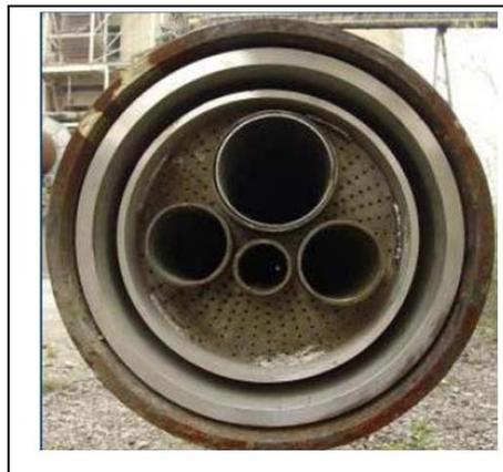
**Figure 1.11:** Example of a multi-channel burner
